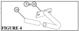
STEP 6:Securely assemble RIGHT (9) & LEFT (10) LEG EXT HANDLES to LEG FRAME (11) using two 3/8 X 4" BOLTS (21), four 3/8" FLAT WASHERS (24), and two 3/8" LOW HEIGHT NYLOCK NUTS (27). See FIG-URE 5.
